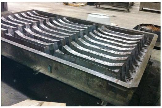
Rebar is placed and tied, in accordance with the structural design. The concrete is then placed in the form and consolidated by external vibration to ensure it has properly molded to the form. The form may need to be topped off after consolidation to ensure that the form is completely filled. Strike off the form to ensure that it is not overfilled.
