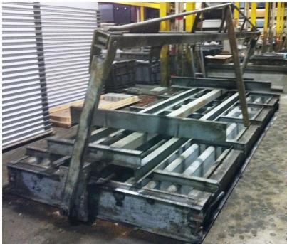
After the product has cured the cattle guard form is then lifted up and the turning latch is disengaged to allow a gravity turn of the form. The cattle guard is then removed from form and the overhead crane takes it to storage.
